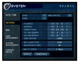
3. Enter the information received in email (including the password). Press the DDNS Status first - wait for the SUCCESS MESSAGE (as long as the information is correct). Select OK to save the settings. The System will restart to activate the new configuration.
